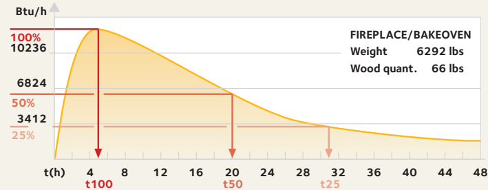
A fireplace reaches peak instantaneous heat release (11942 Btu/h) about 3 hours after heating is started. The fireplace still radiates about 50 percent of its heat output 11 hours and 25 percent 18 hours after heating has started. A bakeoven, which is twice as heavy as a fireplace, reaches peak instantaneous heat release (12624 Btu/h) about 5 hours after heating is started. The bakeoven radiates about 50 percent of its heat output 20 hours and 25 percent 31 hours after heating has started.
